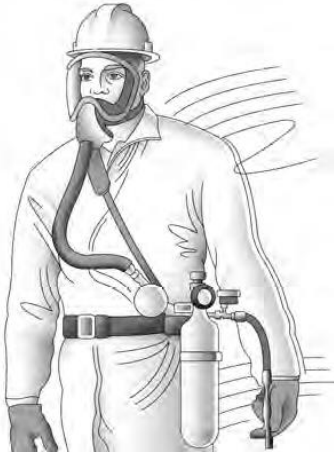
Full Facepiece Supplied-Air Respirator (SAR) with an auxiliary Escape Bottle
