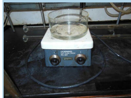
An older model hot plate/stirrer with an oil bath dish (Courtesy University of California, Berkeley)
